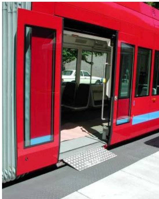
Fig. 7 - Extension of Bridgeplate for Boarding
